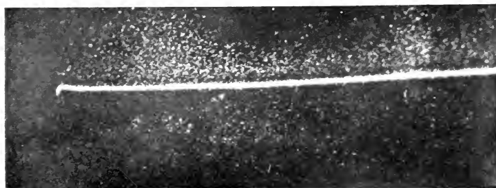
FIG. 126.—Photograph by C. T. R. Wilson of the track of an \alpha particle from radium through air supersaturated with water vapour. [From "Proceedings" of the Royal Society.]
